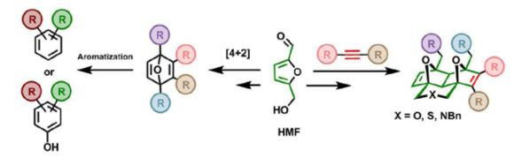
Figure 1. Cycloaddition reactions of HMF derivatives with alkynes.
