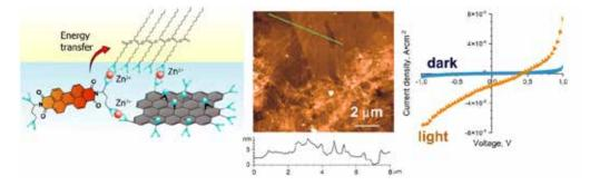
**Figure 1**. Schematically illustrated process of self-assembly of ultrathin hybrid film at air-water interface, AFM image of hybrid transferred onto solids and current-voltage curves of photovoltaic device based on the hybrid measured in dark and under visible light irradiation.
