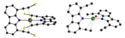
Figure 1. Molecular structures of  $[3,6-tBu_2-1,8-(Me_3SiC\equiv C)_2Carb]_2M$  (M = Ca, Yb, Sm) and  $[3,6-tBu_2-1,8-(PhC\equiv C)_2Carb]_2Ca(THF)$ .
