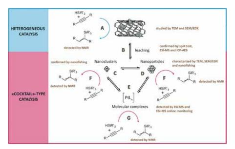
Figure 1. The investigation of platinum catalysed hydrosilylation reaction and methods involved<sup>3</sup>
