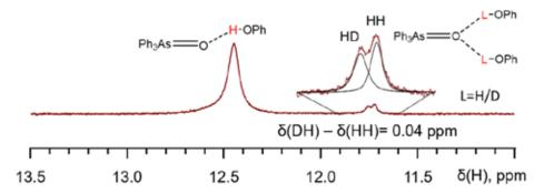
**Figure 2.** The low-field part of the <sup>1</sup>H NMR spectra of deuterated solution (50% D) of Ph<sub>3</sub>AsO and phenol in a mixture of CDF<sub>2</sub>/CDF<sub>2</sub>Cl at 100 K.
