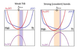
**Figure 1**. The gap width between positions of electrostatic potential minimum and static potential maximum along interatomic line Hal<sup>-</sup>...Tt in Y–TtX<sub>3</sub>...Hal<sup>-</sup> complexes.
