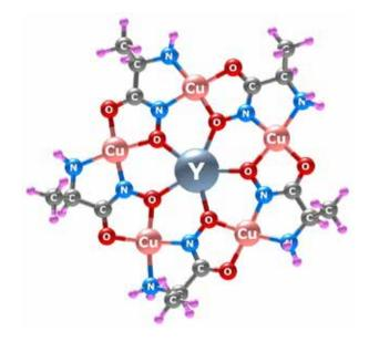
**Figure 1**. DFT optimized structure of the high-spin sextet {Y[15-MC<sub>Cu(II)Alaha</sub>-5]}<sup>3+</sup> complex. Interatomic distances, Å: Y–O(oxime) 2.369–2.394; Cu–O(oxime) 1.945–1.948; Cu–O(carbonyl) 1.923–1.926; Cu–N(imine) 1.890–1.892; Cu–N(amine) 2.022–2.026.
