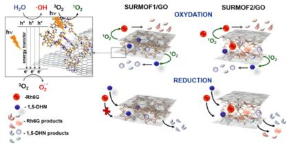
**Figure 1**. Schematic illustration of the proposed size-selective mechanism of photodestruction of Rh6G and DHN in the presence of the SURMOF1/GO and SURMOF2/GO under aerobic and anaerobic conditions.
