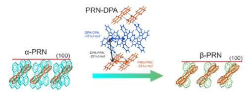
**Figure 1**. Crystal structure fragments of  $\alpha$ -PRN (cyan, sandwich *HB* packing) and  $\beta$ -PRN (green, *HB* packing) in comparison of perylene arrangement in PRN-DPA co-crystal. The structure of co-crystal with interaction energies is illustrated above the arrow.
