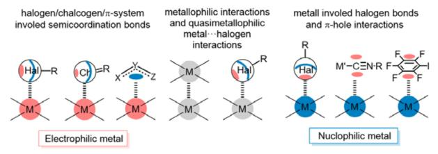
Types of metal-involving noncovalent interaction recognized in [M]-CNRs (M= Pd<sup>II</sup>, Pt<sup>II</sup>) species.
